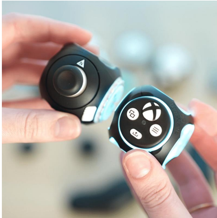
Chart 8: Modular Controller: The Proteus Can be Configured in a Variety of Combinations
