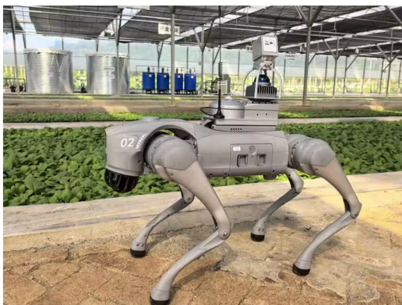
Chart 7: Go2 Quadruped Robot Equipped with Sensors and AI Vision to Monitor Seedling Growth
