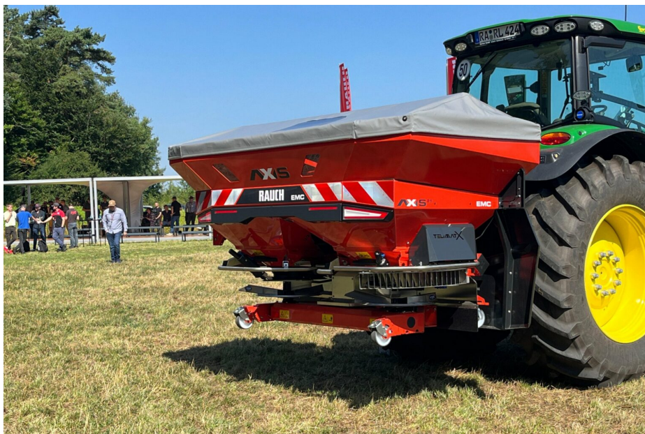
Chart 6: The Axis 25 can Hold 2.5 tonnes of Product, and Spreads up to 42 Metres Wide
