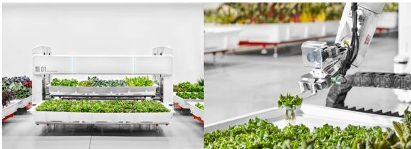
Chart 36: Iron Ox's Self-Driving Robot Angus (Left) and Visual Monitoring System
