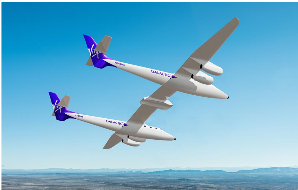
Chart 1: The Mothership is Used to Carry Spaceships up to an Altitude of 45,000 Feet
